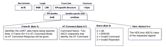
Figure 3-10. AT Command Response Frames.
